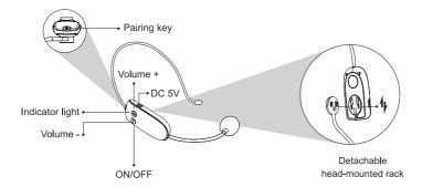
1. The wireless microphone factory setting have been paired successfully, you can use it directly. If the microphone has no sound or the microphone is disconnected, you need to pair it manually.
