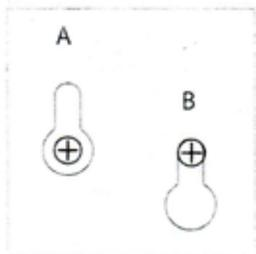
DIVIDERS SNAP INTO SLOTS ON BACK OF POCKET. WITH THE LARGE TAB ON TOP, SET TABS IN BACK SLOTS AND TWIST INTO PLACE.
