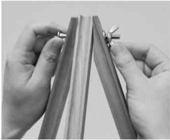
4. Thread the 2nd longest wing-nut and screw through all 3 legs at the top. The 2 angle cut legs rest flush against the back leg.
