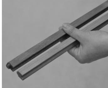
2. Select a bottom leg and a top leg. Bottom legs have feet on the end and nest into the groove of the top legs.
