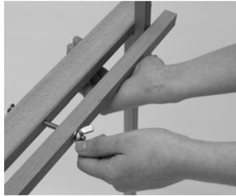
5. Clamp the tray over the front legs using the longest wing nut and screw, and tighten.
