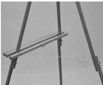
7. Attach the other end of the chain with hook, to the back leg.
