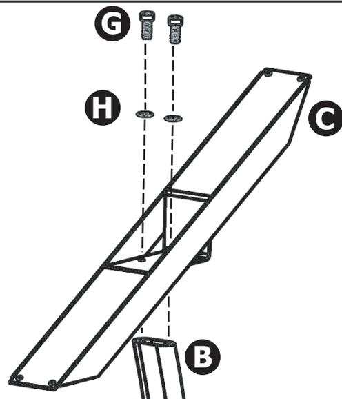
Attach mounting bracket to post using M8 socket head screws and washers. Use supplied hex key.
