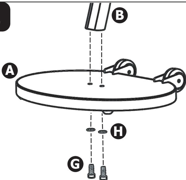
Attach post to base using M8 socket head screws and washers. Use supplied hex key.
