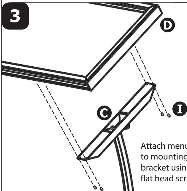
Attach menu board to mounting bracket using M4 flat head screws.
