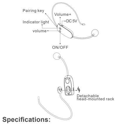
Microphone: Unidirectional condenser microphone
