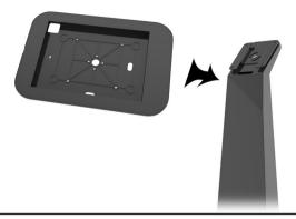
3. Unlock the cover and take out the panel diagonally.
