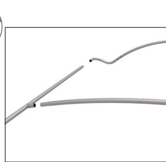
3. Make sure that the middle support is fitted into the frame.
