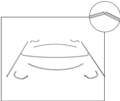
1. Assemble the two long curved and long straight sections.
