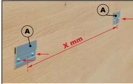
2. Screw the Z-brackets to the wall. Wall anchors are provided if mounting on to concrete wall. Distance between the brackets (X) should be equal to the distance between the mounting plate on the back of the notice board (Y).
