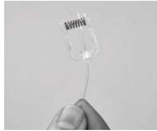
3. Tie fishing wire to the bottom half of the ceiling fitting.
