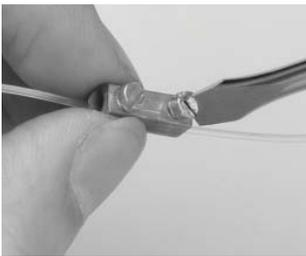
6. Slide the grip into desired position. Tighten the grip onto the wire using a screwdriver.
