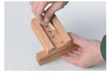
10 Place the cover plate in guide holes covering the screw
