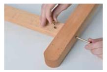
**2** Flip it over and bolt the parts together
