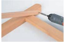
Screw the support rod to the base
