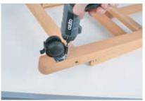
Screw on the wheels onto the base of the easel.
