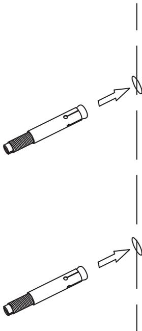
Knock the dynamolts into the wall until the flange is flush to the wall surface.
