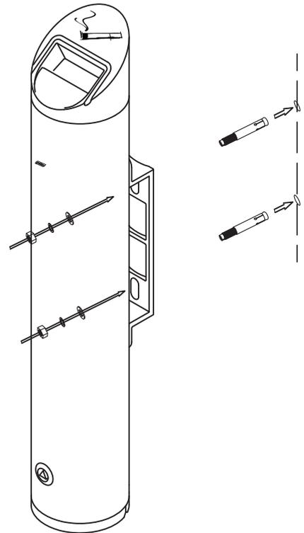
Mount the ashtray onto the dynamolts and tighten the nuts using the wrench provided.
