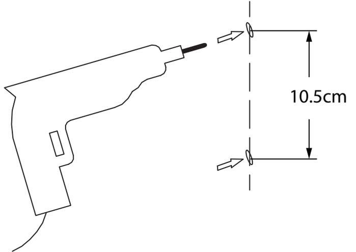
Mark the position of the holes at 10.5cm apart on the wall
