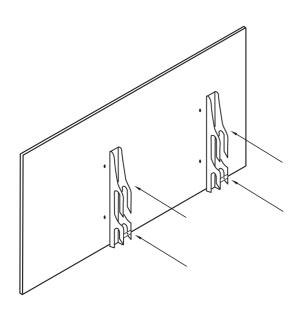
**Step 6.**Mount Brackets (E) into the back of LCD screen.
