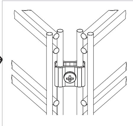
2. Place 3rd Grid panel on base, then Connect both sides to the first 2 panels as shown in Step 1.
