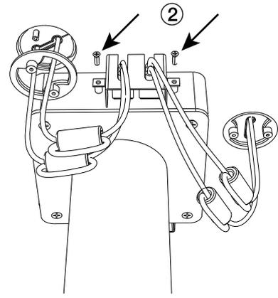
② Unscrew the 2 screws on cable cover.
