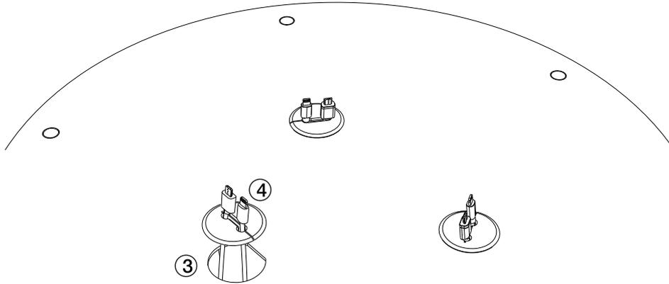
③ Remove cables from cable clip.
