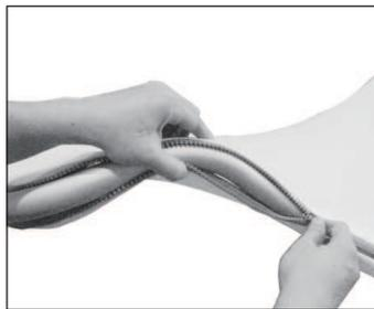
6. Zip the bottom edge of the graphic beyond the centre point as shown above. Zip the remaining side and bottom to meet at the corner.
