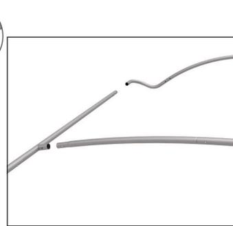
3. Make sure that the middle support is fitted into the frame.
