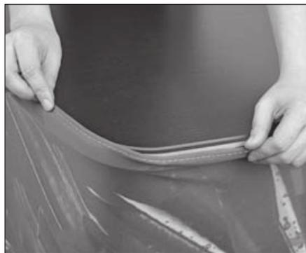
5. Tuck the edge of the fabric into the groove of the table top to secure.
