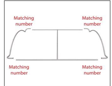
4. Connect corner sections to straight sections by matching the numbers.
