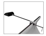
7. Attach lights as desired and tighten the clamp to hold into place.
