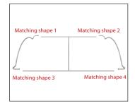
4. Connect corner sections to straight sections by matching the shape codes.
