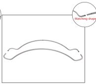
2. Connect corner sections to curved sections by matching the shape codes.
