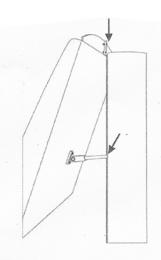
Slide the support arm (attached to the shelf) and the connector plate into the pole groove
