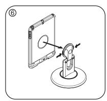
Press buttons, attach shell, release buttons, and spin until you hear the click
