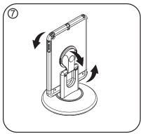
Rotates 360°, tilts for angle adjustment, and reversible view
