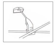
6. OPTIONAL Attach lights to top of the frame by sliding the plastic X-Blocks under the frames cross sections.
