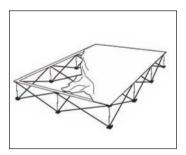
4. Work continuously in one direction accross the frame until the graphic entirely covers the frame.
