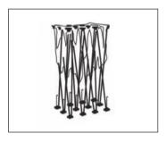
1. Remove the frame from the protective case and place on a clean flat surface with the velcro on the top.
