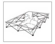
3. Starting on one side, attach the velcro side of the graphic to the velcro on the frame. Overlap velcro of graphic about 6mm on all sides on the velcro on the frame.
