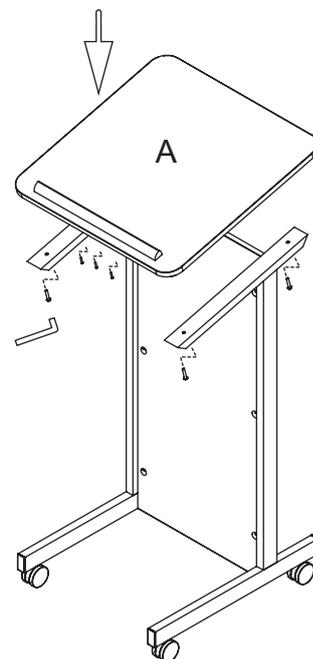
Fix the Top board to the frame using the bolts provided.
