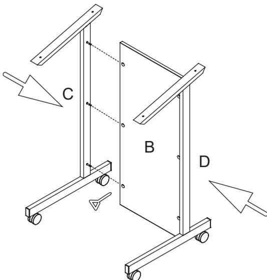
Assemble the Rails onto the Back board.
