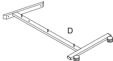
Assemble the rails. Screw in the cam bolts and castors on to the metal frame.
