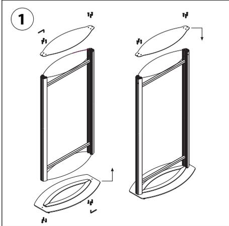
Screw the bottom and the top plate to the side columns of the light box
