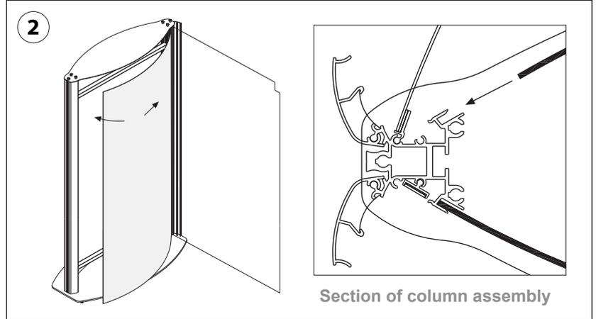
Place the full length plastic diffusion panel and clear plastic lens into the channels on the side columns (as shown in the detail drawing) ensuring that the decorative panel is at the bottom of the display
