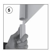
Take the remaining two Header Tubes (G) and insert the tapered ends into the tubes on the Header Card (F)
