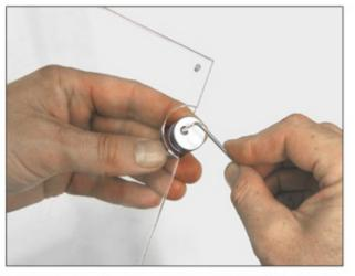
Slide the cut-out areas of the acrylic into the slots on the stand-offs. Centre the stand-offs in the cut-out area and loosely fasten the grub screw as shown
