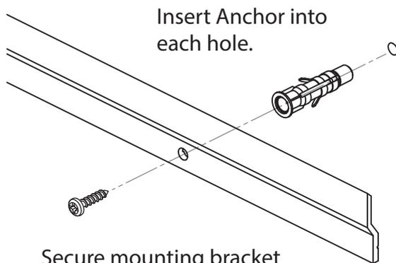
Secure mounting bracket to wall using supplied screws. Use minimum 5 screws per bracket. Mounting bracket must not be loose on wall.
