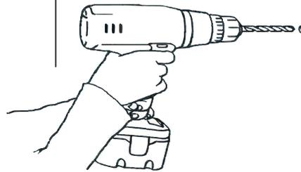
Drill hole in to wall at each location.
