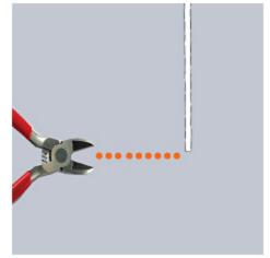
Measure the Cable and pull taut, then using cable cutters or pliers, cut the Cable to desired length.
