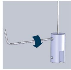
3. Reattach the Panel Holder to the Cable and tighten the Grub Screw.
