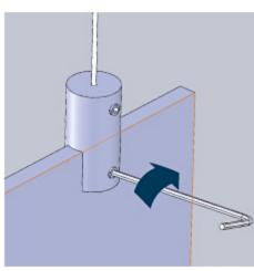
Loosen the Grub Screw on the Panel Holder and place your panel into the holder. Then tighten the Grub Screw to secure the panel to the Panel Holder.
