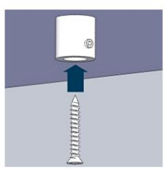
4. Fasten the Ceiling Anchor to the ceiling using the screw provided.
