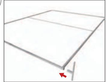
4. Connect feet to the frame by pressing & pushing.
