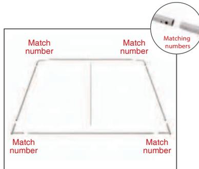
2. Connect corner sections with matching shape codes.
