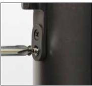
Insert the new cartdridge and screw back onto the post
