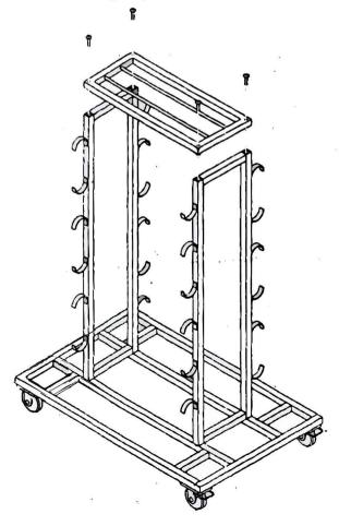
2. Put the two side frames on the under frame and screw them tightly.
