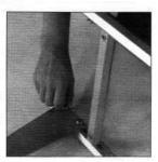
•Screw and fasten the legs on the main body profile of the frame.
