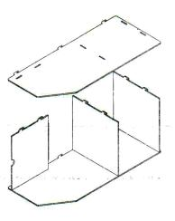
STEP3. Install the back plate and put it into the clamp position.
