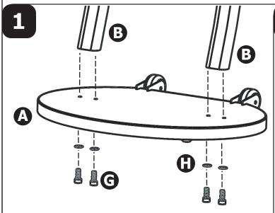
Attach posts to base using M8 socket head screws and washers. Use supplied hex key.
