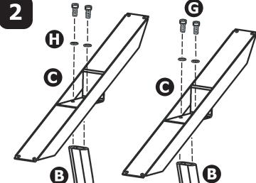
Attach mounting brackets to posts using M8 socket head screws and washers. Use supplied hex key.
