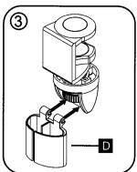
Attach part D to the assembled component.
