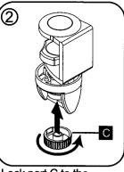
Lock part C to the assembled component.
