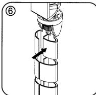
Hold down one side of part D to open a slot.
