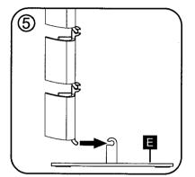
Attach part E to the bottom of the chain.
