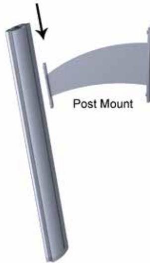
2. Tighten the grub screws to fix the post at the desired height using the allen key provided
