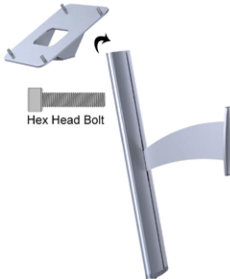
4. Screw the holder to the wall. Use the plastic wall plugs when securing to concrete.
