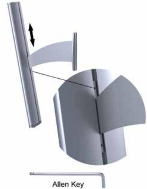
3. Secure the top bracket to the post with the bolts provided
