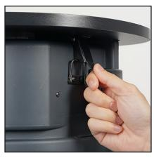
3. Secure 4 underside latches to hooks attached to shipping case.
