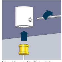
Insert the end of the Cable with the Cable Stop into the Ceiling Anchor and fasten both Grub Screws.
