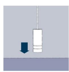
Allow the Floor Coupling to hang on the Cable. It should come to rest just above floor level.
