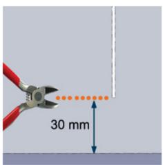
4. Pull the cable taut to the floor and trim it at a height of 30mm above floor level.
