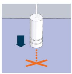
7. Mark the floor directly below the point at which the Floor Coupling rests.
