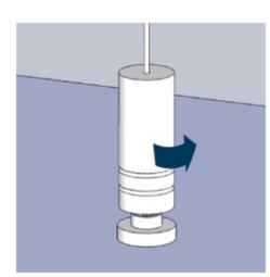
Screw the Floor Coupling onto the Floor Anchor until the Cable is taut.
