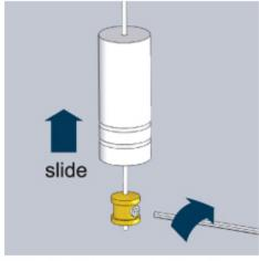
3. With the Cable suspended from the ceiling, loosen the Grub Screw on the Adjustable Cable Stop. Slide the Adjustable Cable Stop and Coupling up the Cable until it is above the level of the floor, then loosely fasten the Adjustable Cable Stop.
