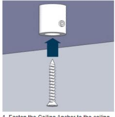
1. Fasten the Ceiling Anchor to the ceiling using the screw provided.
