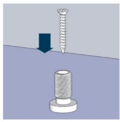
At the point you have marked, fasten the Floor Anchor to the floor using th screw provided.
