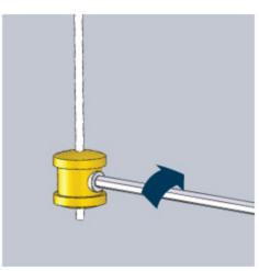
5. Loosen the Grub Screw on the Adjustable Cable Stop and slide it along the Cable until it reaches the end. Tighten the Grub Screw firmly to fasten the Adjustable Cable Stop at the end of the Cable.
